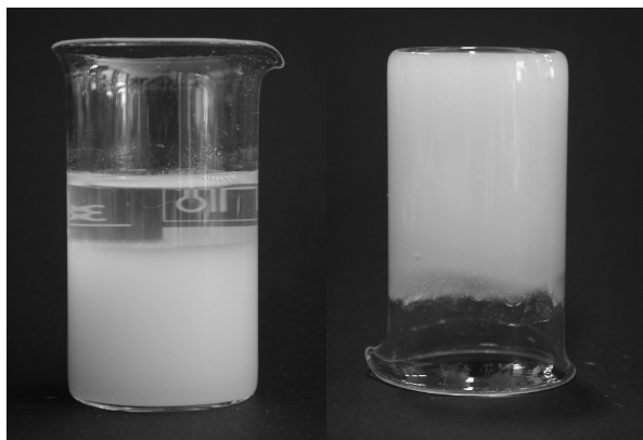
Figure 2. A 2% aqueous suspension of cell wall material from the parenchymatous tissue of ripe fruit. Left: before shear. Right: after shear.
